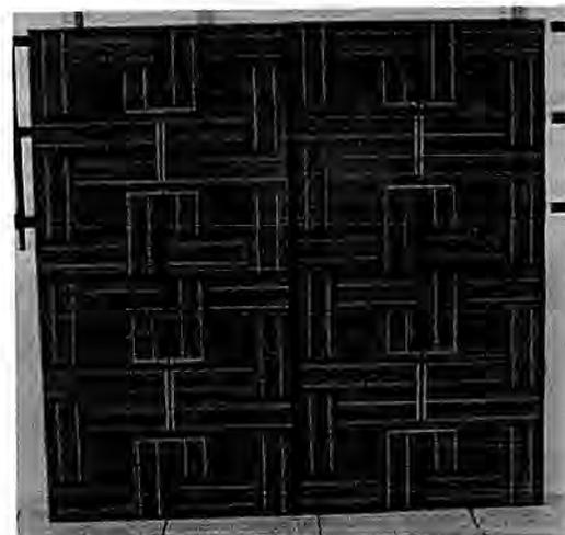
Figure 4: Loop-Antenna PV module
