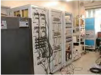
**Figure 5:** The reduced scale distribution system simulator.
