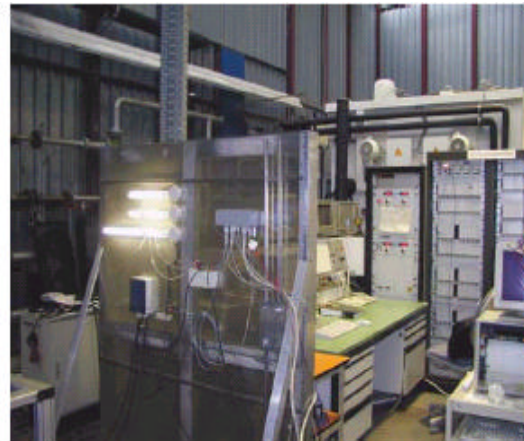
Figure 5: a) Test set-up for system testing of an SHS b) Installed SHS tested in lab of TÜV Rheinland
